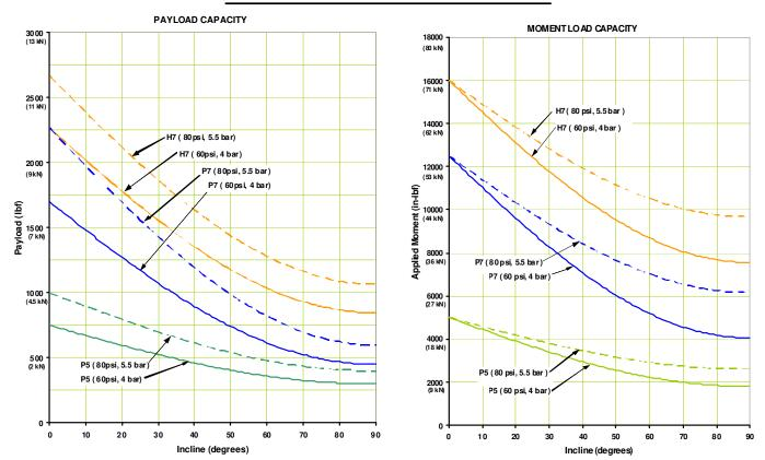
Applications are evaluated in two seperate calculations: payload and moment load. An approvable application meets both criteria. For applications outside the graph safety zone, contact Welker.
