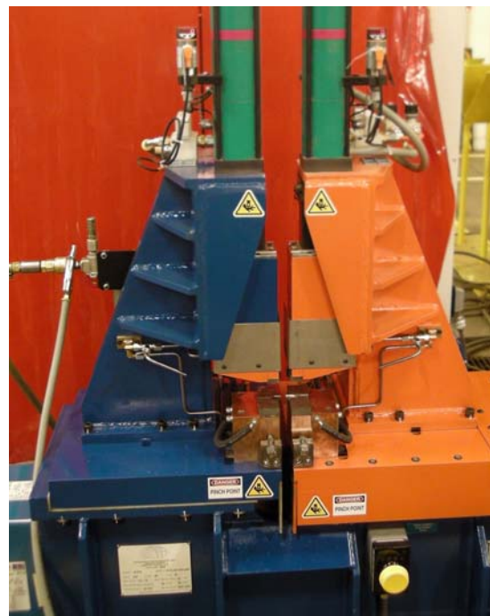
Bonded gib slides for flash welding application: automotive battery terminals to cables
